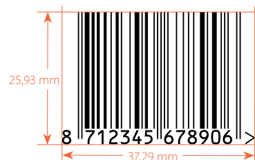
The nominal dimensions of the barcode (100%)
