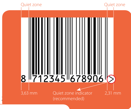
The dimensions of the quiet zones in the nominal EAN13 symbol
